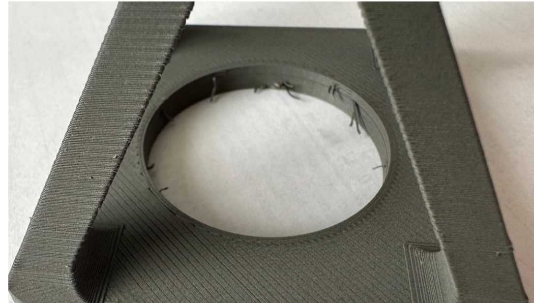
Stringy defects on the inner ring of the pyramid
