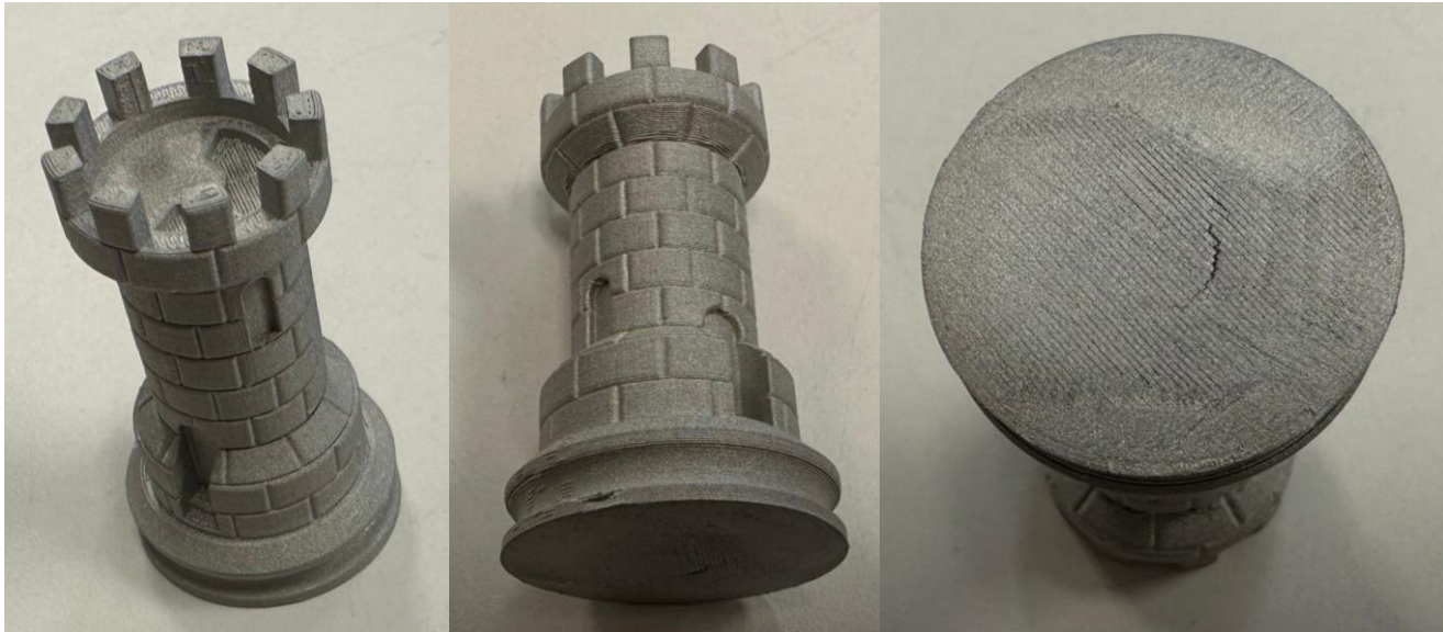
Views of printed part, minor crack in bottom
