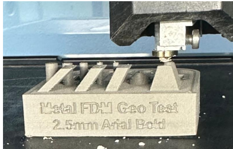
Near-finished print, notice warping and crumbs
