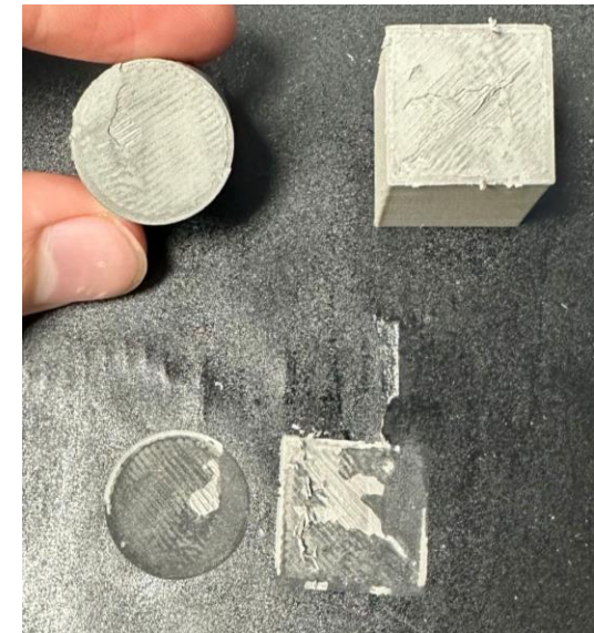
Part removal residue on build plate
