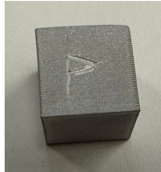
MakerBot Print Cube Ideal top and stringy bottom layers
