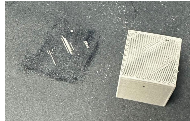
Removed print with stringy first layer, indicating too far away from build plate
