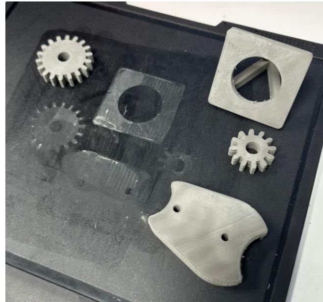
Print residue left on print bed
